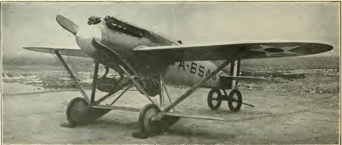
The Navy-Wright plane, equipped with Wright T-2, 12 cylinder engine. The first complete airplane of the Wright Aeronautical Corporation
